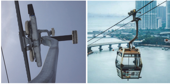
Figure 2 detachable grips on a chairlift and bicable gondola [10, 11]
