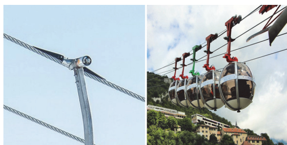
Figure 1 Fixed grips on a chairlift and pulsed gondola [8, 9]
