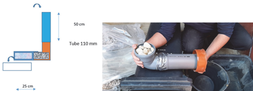
Figure 2 Filtration test setup used for materials 0-4 mm and 0-32 mm
