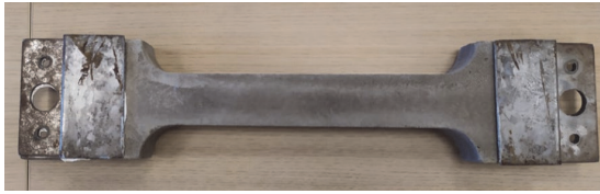
Figure 2 The test specimen of foam concrete FC-500
