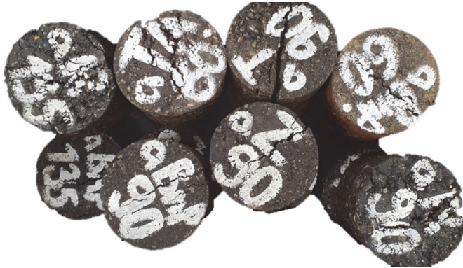
Figure 2 Test specimens after indirect tensile strength test
