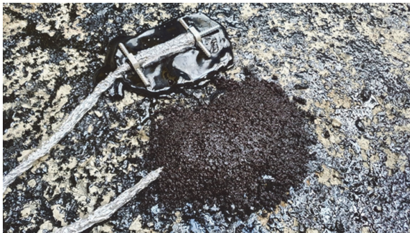
Figure 4 Horizontal strain sensors KM-100HAS designed for asphalt layers
