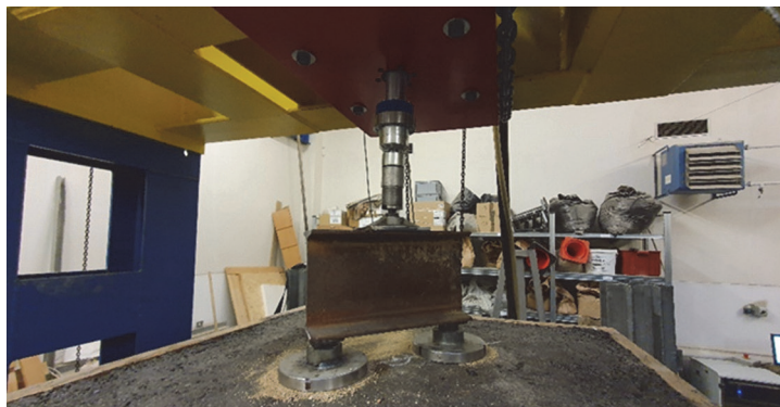
Figure 2 Full-Scale model - load plates, spreader beam, hydraulic press
