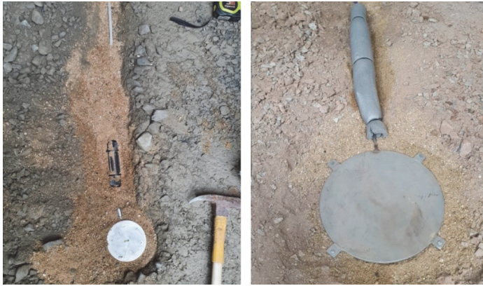
Figure 3 Pressure gauge boxes TML KDC-500 (left) and GEOKON 3500 (right)
