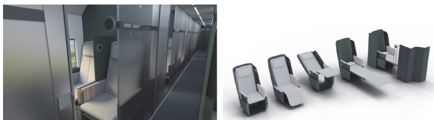
Figure 3 Private compartments with pull-out bed function & modular seat design (© moodley)
