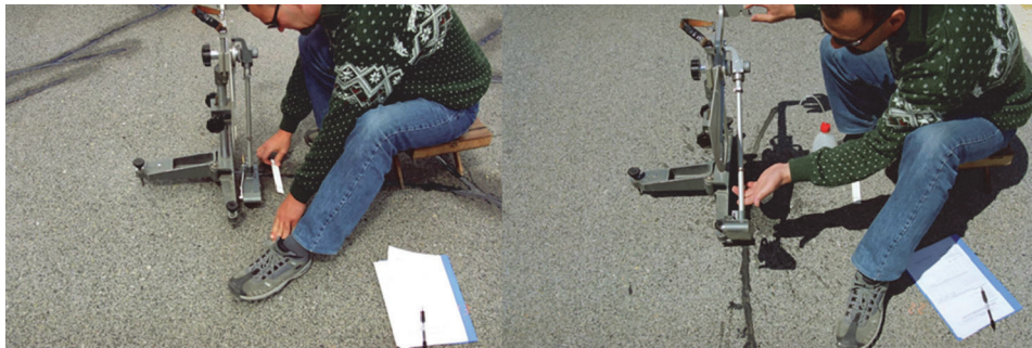
Figure 3 The SRT was used to measure directly on the sealed crack in both the transversal and longitudinal direction
