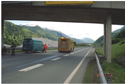
Figure 2 The SCRIMTEX device was used to measure the average effect on the overall skid resistance of the entire road surface
