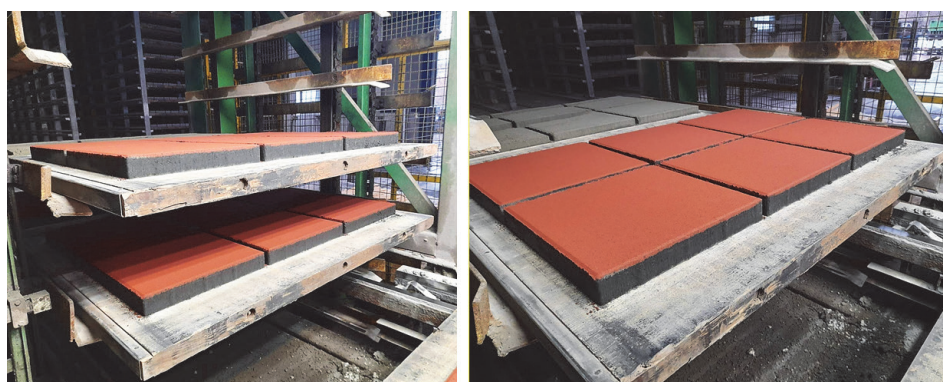
Figure 1 Fabrication of precast prototype concrete slabs incorporating SSA within an industrial setting
