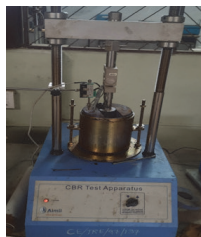
Figure 7 CBR test on sample
