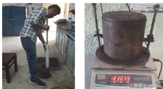
Figure 6 Compaction of sample for modified proctor test
