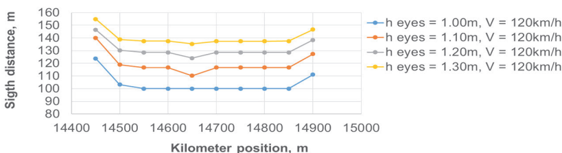
Figure 11 Sight distance as a function of kilometeric position, for speed 120 km/h and h_{\text{obstacle}} = 0.00 \text{ m} , on vertical convex curve area – horizontal alignment
