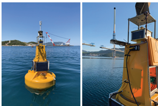
Figure 3 Measurement buoy with construction activities in the background (Photo: Alan Blažekovič).
