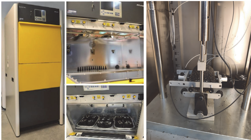
Figure 3 Atlas Sunset XXL solar conditioning unit (left), configuration for stiffness modulus measurement (right)
