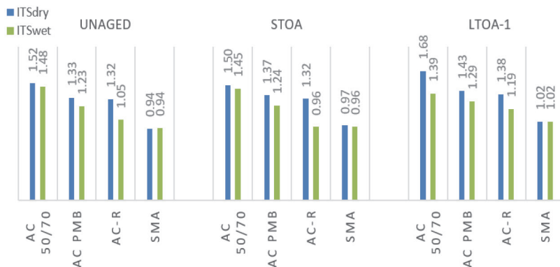
Figure 6 Indirect tension strength of dry and wet specimens of unaged and aged tested mixtures
