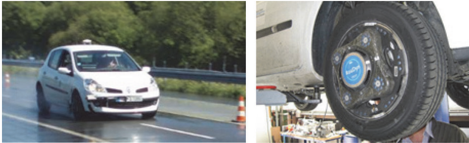
Figure 6 Instrumented Clío 3 Setup for Braking Tests
