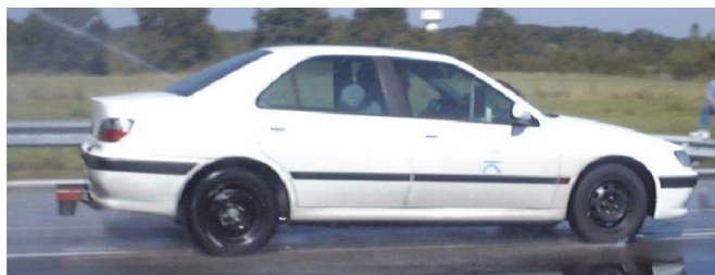
Figure 1 Test vehicle “406” on the test track (Correvit sensor at the rear)
