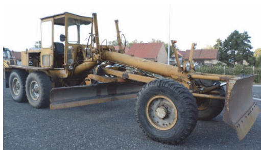
Figure 2 A grader used by Hungarian Public Road Non-Profit Liability Company (Photo: Csaba Tóth)
