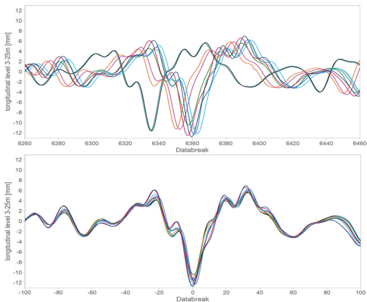
Figure 2 Longitudinal level before (top) and after (bottom) the repositioning process
