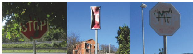
Figure 1 Examples of some of TSRS challenges - occlusion, damaged sign, faded sign with graphic changes
