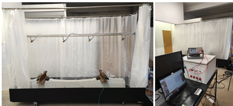
Figure 2 Specimen prepared for testing the electrical resistance (left), equipment used for the measurement (right)
