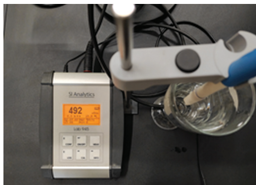
Figure 4 Measuring the electrical conductivity of water using the conductometer SI Analytics Lab 945
