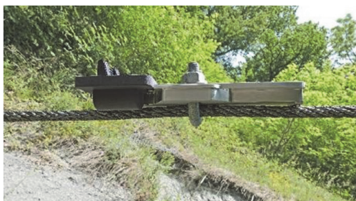
Figure 3 Guiding the rope along the Guard and the wire rope clamp, allows measurement of the force in the rope
