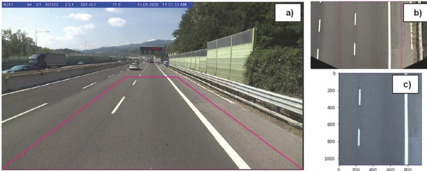
**Figure 1** Pre-processing of the images: a) the original ARAN image with the area of interest; b) orthogonal projection of the area of interest; c) final image (dimensions in pixels)
