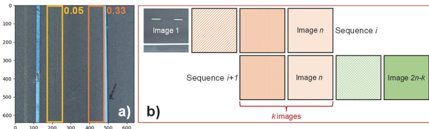
**Figure 2** Image analysis: a) example of two potential top-down cracks with different prediction confidence levels; b) image sequences (scheme)
