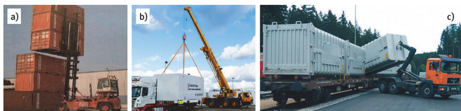
Figure 1 a) Mast forklift truck for moving containers [2]; b) Reloading of a container using a mobile crane [3], 1c) Reloading of a container using the ACTS system with the hook-type equipment [4]
