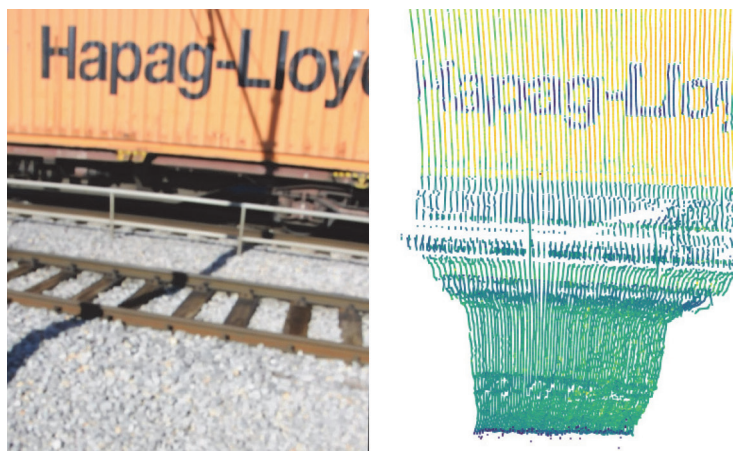
Figure 7 A container with inscription (left) and its recognition with the reflectivity measurements performed by the OS1 LiDAR sensors (right)
