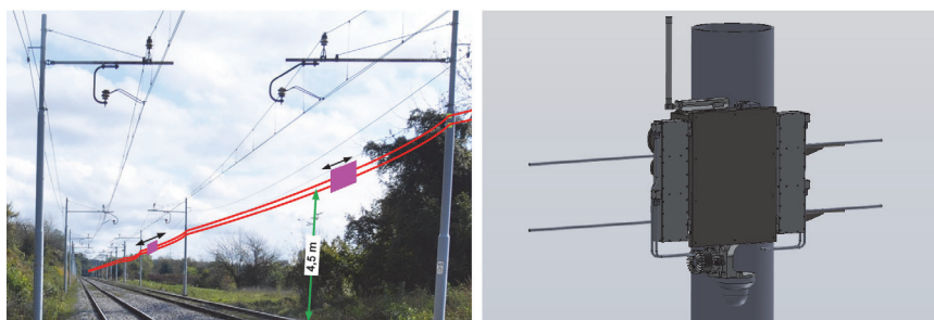
Figure 6 InspectRail concept: LiDAR sensor mounted on an autonomous mobile robot that moves along wires on the catenary poles
