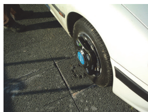
Figure 2 The Kistler wheel on the MEVI system [6]
