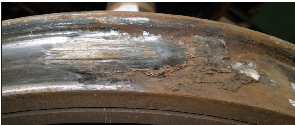
Figure 4 Effects of speed and higher axle loads
