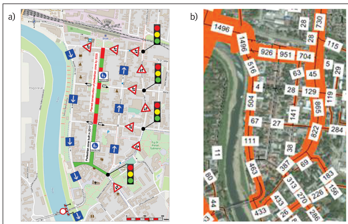
Figure 4 a) The plan of the traffic flow regulation, Sisak 2025; b) Traffic load in the afternoon peak hours, Sisak 2025
