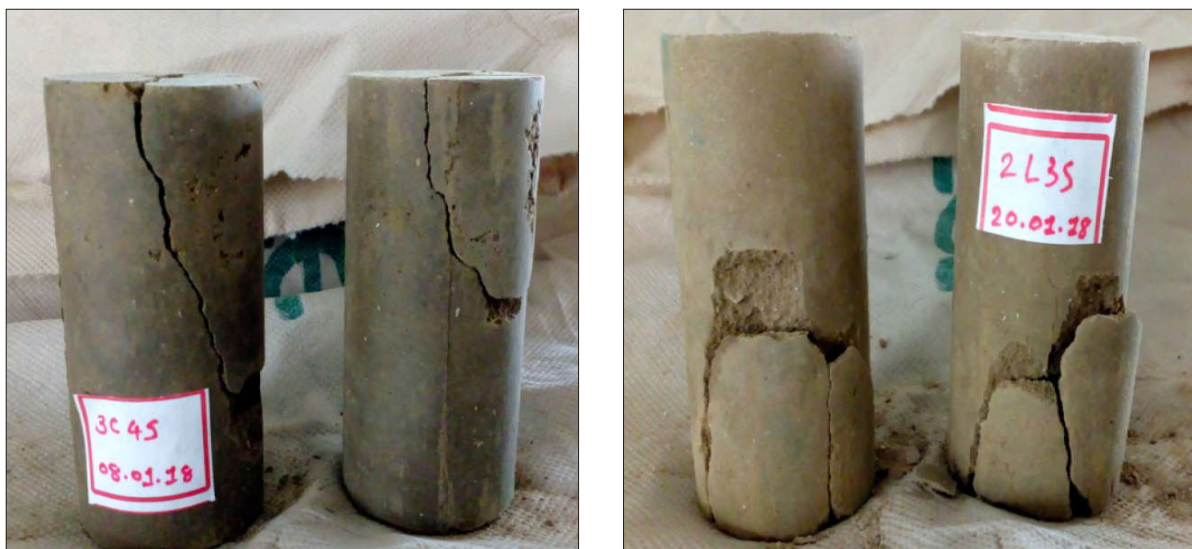
Figure 7 Failure Pattern observed in 3C4S and 2L3S
