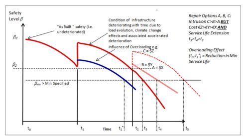
Figure 5 Probabilistic life cycle optimization model integrating condition monitoring information
