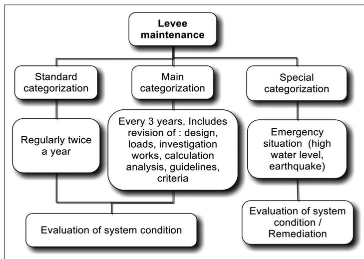
Figure 2 Guidelines for frequency of levee assessment [1]
