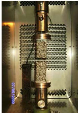
Figure 2 Uniaxial Tensile Strength Test – UTST (left) and longitudinal crack at the wheel tracks (right) [3]
