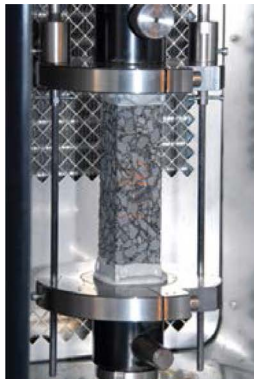
Figure 1 Tensile Stress Restrained specimen Test – TSRST (left) and transversal thermal crack (right) [3]
