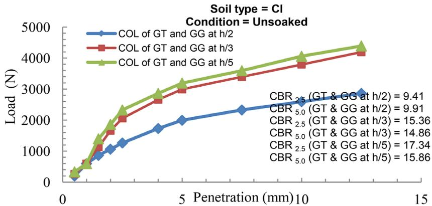
Figure 5 Load v/s penetration curve for COL for various positions of GG and GT
