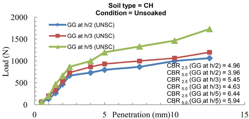
Figure 3 Load v/s penetration curve for SIL of GG at different position (UNSC)
