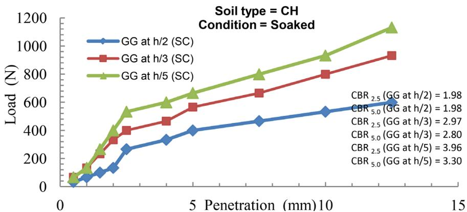
Figure 4 Load v/s penetration curve for SIL of GG at different position (SC)
